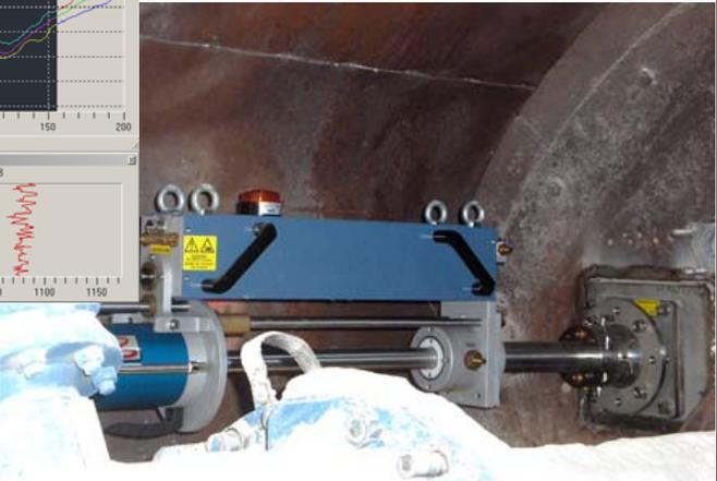
**Installation on kiln hood wall**
